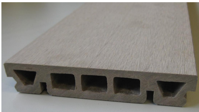
Figure 1: Example of WPC decking profile DURO.
